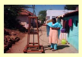
A mobile RF drive test measurement cart carrying the measuring equipment along with antennas and amplifiers is used for carrying out the measurement. The building losses due to different kinds of building materials and path loss are measured using the measurement system in certain selected villages. The data is then used for building up a seamless wireless connectivity for rural parts
