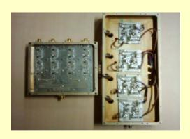
The localization is done by using two sets of RF phased array front-end modules. The major responsibilities include the designing of the phased array antennas with can radiate a pencil beam of a very narrow beam width, a two bit phase shifter with control modules and the power dividers. The simulation was done using ADS 2002C and fabricated on a glass epoxy substrate. The modules were tested for performance using Network Analyzer.
