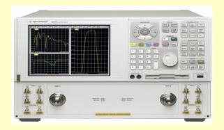
The Agilent PNA-L vector network analyzer is a member of the PNA series network analyzer platform and is designed for general-purpose network analysis needs.
