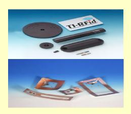
The Tag it Smart labels are a part of the series 6000 family and are designed for tracking and managing thousands or even millions of items with quick, accurate, and non line of sight identification. The TI – RF ID systems offer two versions of smart labels. The tags operate at the frequency of 13.56 MHz
