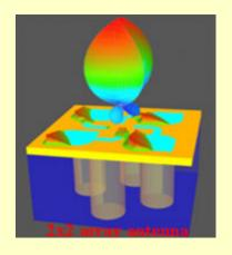
Empire is a versatile 3D Electromagnetic Field simulator developed by **IMST**, **Germany**. It is based on FDTD (Finite Difference Time Domain) method, which has become a standard in RF-component design. EMPIRE is a Electro Magnetic field solver for the analysis of Packages Interconnects, Radiators and waveguide Elements.
