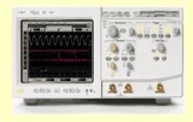
The Agilent Infiniium 54833A is a 1 GHz analysis oscilloscope. It has a 1 GHz bandwidth and a sample rate of up to 4 GSa/s ensuring fast, accurate capture of waveforms.
